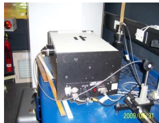
Figure 2.3 Optical bench of Glen spectroradiometer consisting of detector, input optics and fibre-optic cable
