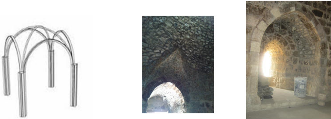
Figure 22. Groin vault, can be thought of as the intersection of two barrel vaults
