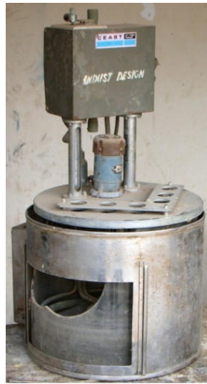
Plate 4: This Density Comparator is obsolete and completely broken down.
