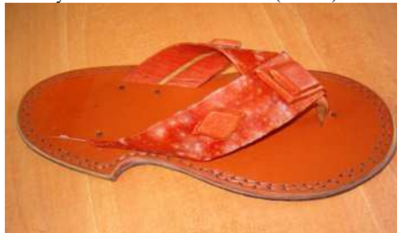
Plate 3. Mouldy leather article, 'Traditional Slipper'
