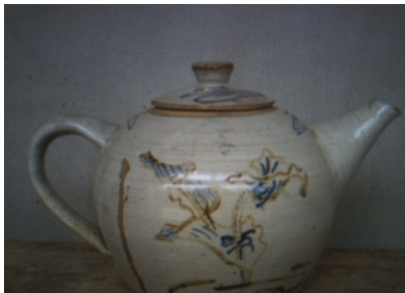
Plate 13: Opacified glazed samples produced using tin oxide with transparent glaze.
