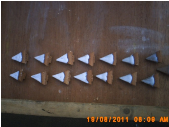
Plate 13: Opacified glazed samples produced using tin oxide with transparent glaze.
