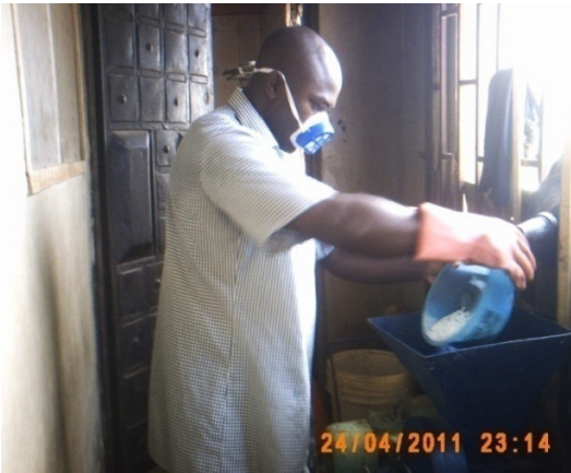
Plate 7: Grinding of the bones
