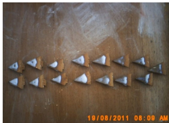
Plate 12: Opacified glazed samples produced using Cow bone ash with transparent glaze.
