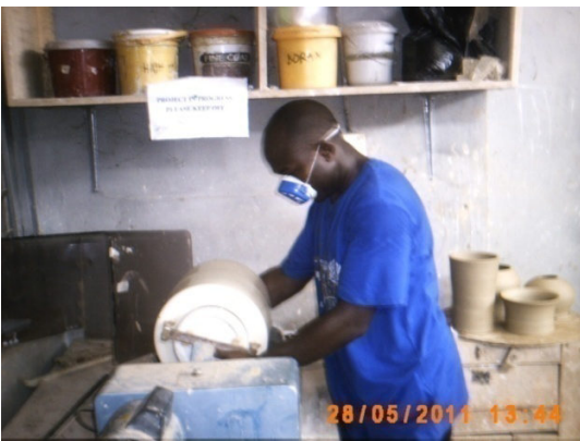
Plate 9: Placing the jar on ball mill machine
