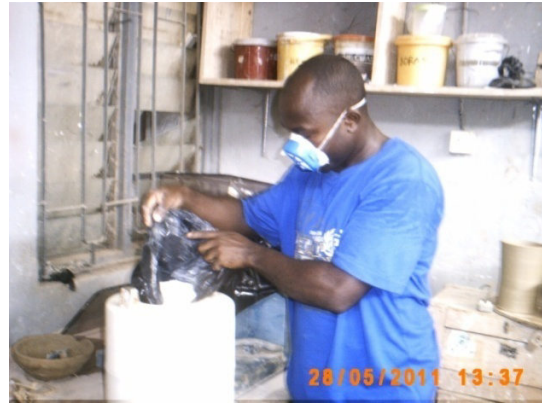
Plate 8: Charging of bone into mill jar
