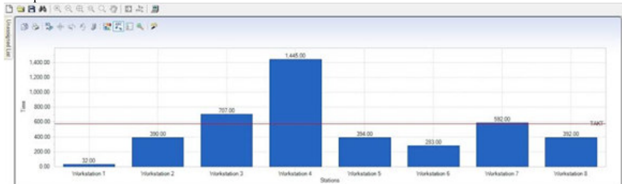
Figure 2: Station line view with a cycle time of 576seconds (using MATLAB software)
