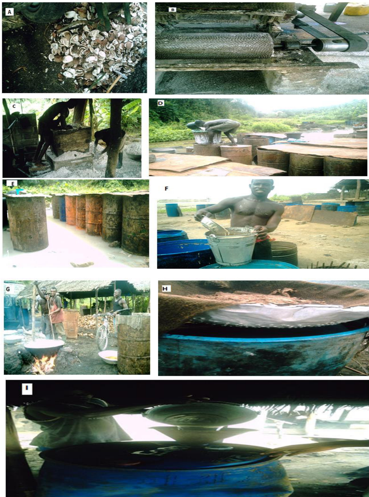
Figure 2: Plates showing the various processing operations; 2A; Coconut meat removed from the shell for crushing, 2B; Rotary Grater used for crushing the meat 2C; crushing of the meat, 2D; mixing crushed meat with water to obtain milk, 2E; settling/fermentation process 2F; skimming suspended oil from water surface after settling, 2G; drying/boiling process, 2H; filtering cooled oil after drying, 2I; storage of coconut oil in large plastic containers
