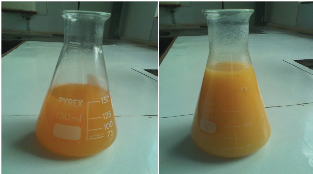
Fig. 2: Molten Nile perch ( Lates niloticus ) viscera oil. Crude (left) and high melting point (right) fractions
