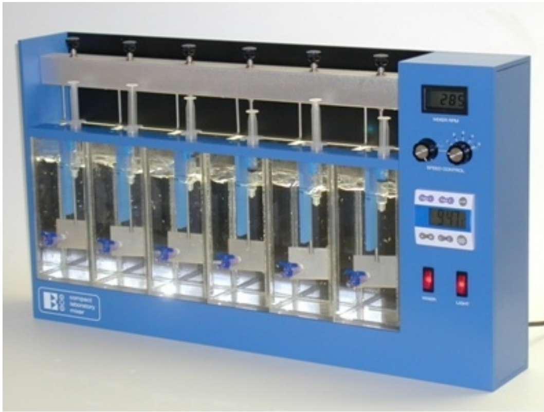
FIGURE1 FLOCCULATOR FOR JAR TEST.
