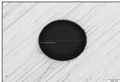
Fig. 3a: the diameter of Nozzle #1 before spraying with tap water.
