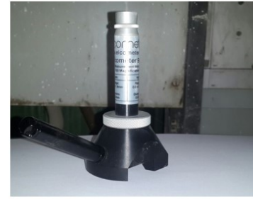
Figure 5. Concrete crack microscope
