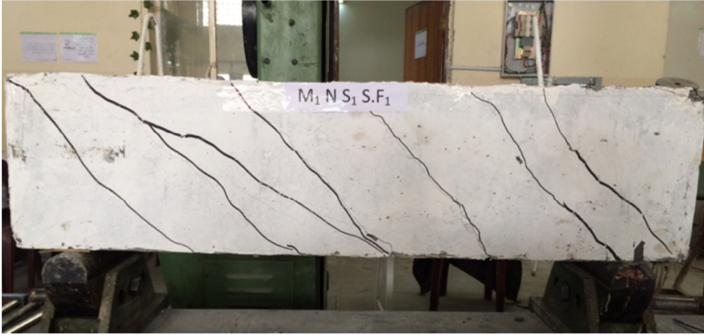
Figure 5. The failure mode for the beam ( M_1NS_1SF_1 )
