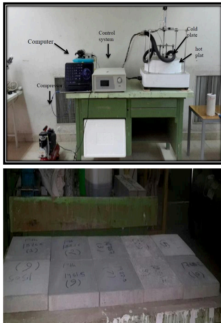
Figure 3. Thermal Conductivity Machine and Specimens of Test
