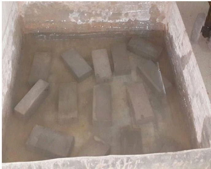
Figure 2. Water Absorption Test for LWFC Bricks
