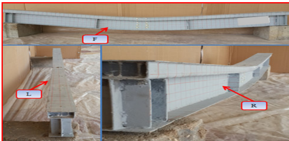
Figure13: Failure of Beam TF40 after Testing.
