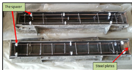
Figure 2. Details of the steel mould of column specimens.
