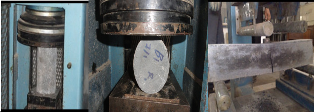
Figure 5. Compressive Strength ( f_{cf} ), Tensile Strength ( f_{sp} ) and Modulus of Rupture Tests
