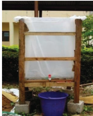
Figure 2: Wetland Unit with Lining
