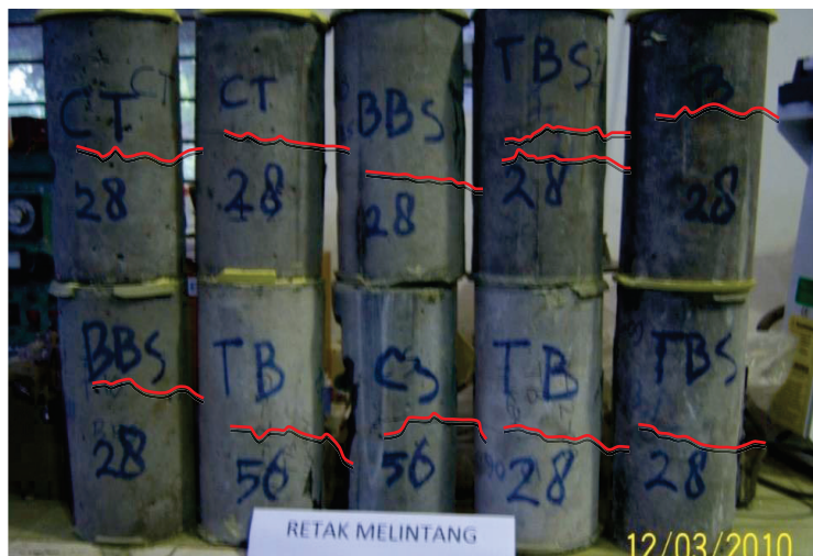
Fig. 5. Compression failure type of specimens with superplasticizer H
