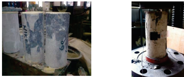
Fig. 4. Compression failure type of specimens with superplasticizer V
