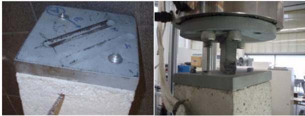
Figure 2 Load reception plate & application of the load to the top of the column
