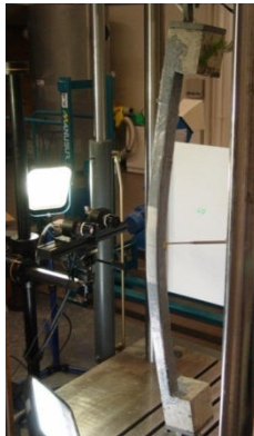
Figure 3 : Column during test.
