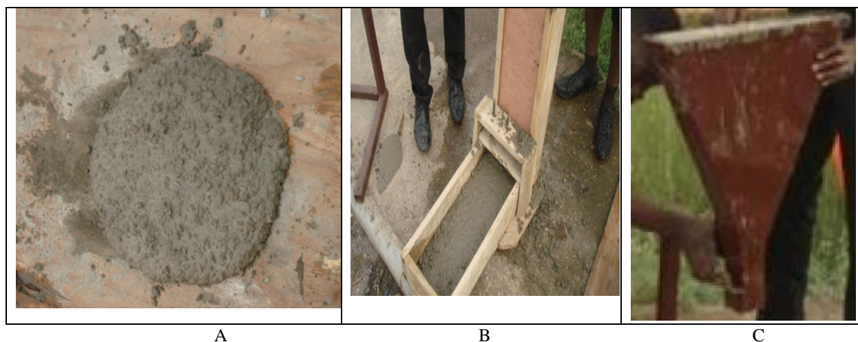
Figure 2: fresh SCC test execution. A) slump spread; B) L-box test and C) V-funnel test.
