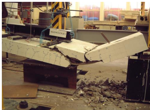
Fig. 5. Shear failure of SG13-9-2 under mechanical load.
