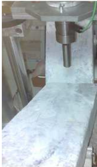
Figure 2. The experimental impact flexural test rig.
