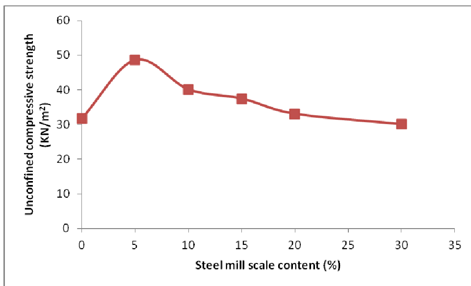
Fig.9: Variation of Unconfined Compressive Strength with Steel Mill Scale content for the soil samples
