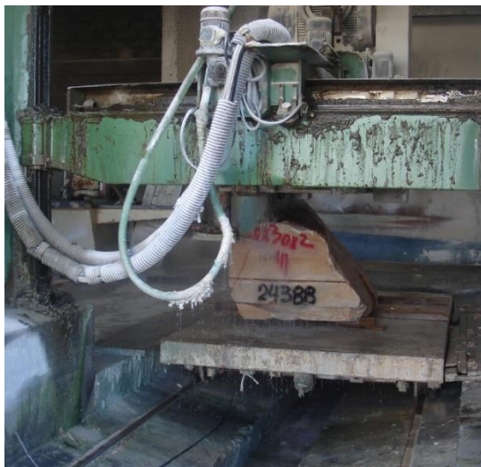
Figure 1 – Primary cut of a marble block in processing industry.
