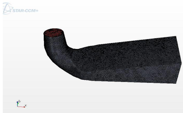
Fig.3.MESH MODEL OF DRAFT TUBE
