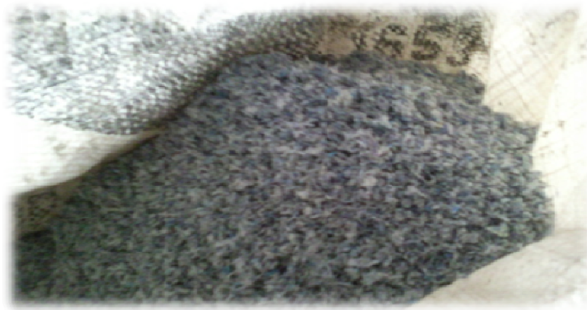
Figure 2 Shredded PWS used for modification
