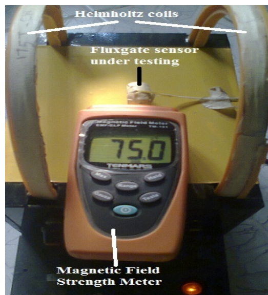
Figure 4: Helmholtz Coils Characterization used as a Test Bed for testing FMS.
