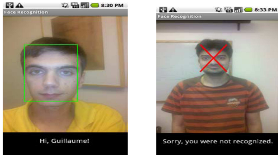
Fig. 4 Result of the Face Recognition application for Android. (a) Client correctly recognized, (b) Client correctly rejected [5]
