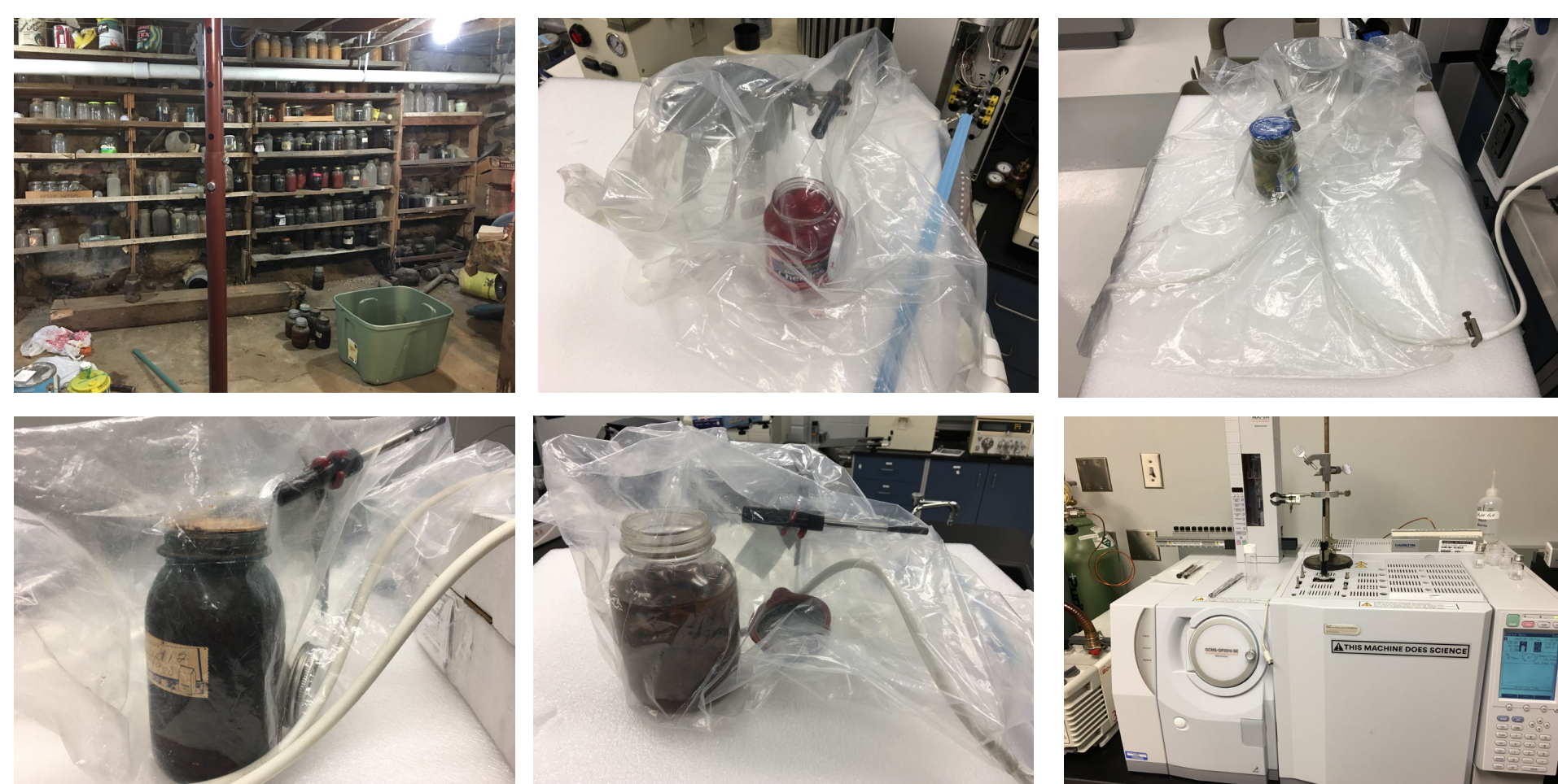
Figure 1. Representative images of the late 19 th century-constructed basement housing the early 1950s preserves, SPME sampling of store-bought preserves and 1950s preserves inside the argon-filled AtmosBag, and direct injection of the SPME device into the GC-MS for analysis of sampled volatiles.
