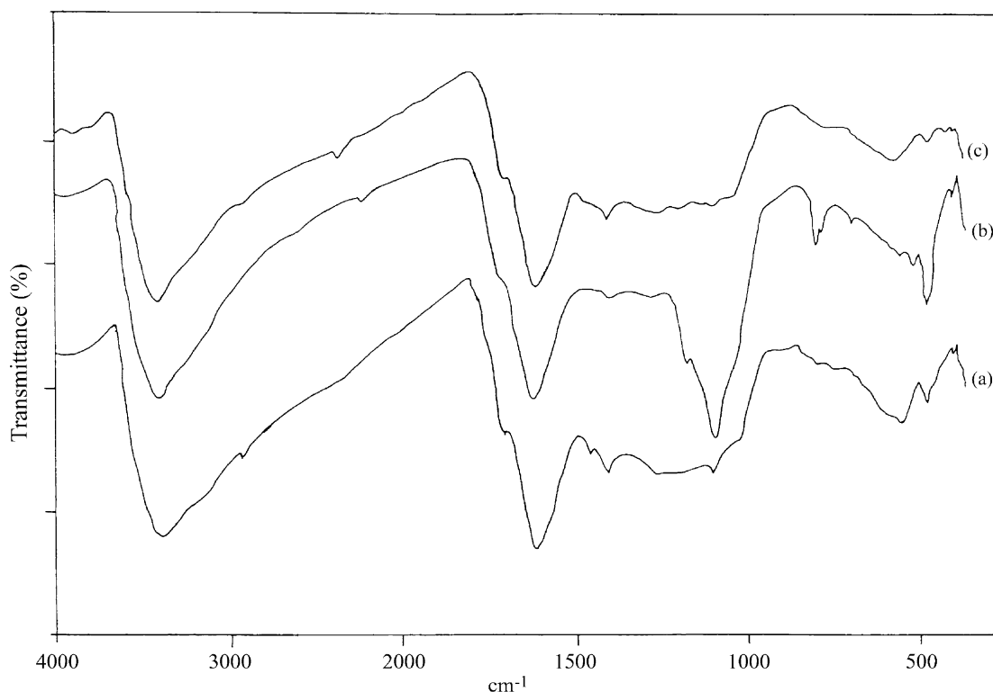
Fig. 1. Infrared Spectra of Tirap coal (a), Tikak coal (b) and Boragolai coal (c).
