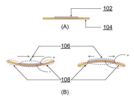
Fig. 1: Operation of a piezo buzzer, and proper placement of a slotted antenna therein
