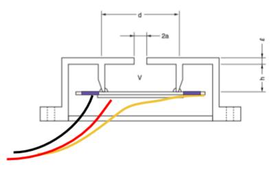
Fig. 4: Placement of the slotted antenna within a nodal-supported piezo buzzer
