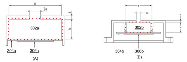
Fig. 3: Piezo buzzers within their cavity resonators, and proper placement of the slot antenna
