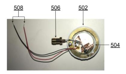
Fig. 5: A wireless antenna integrated with a piezo buzzer
