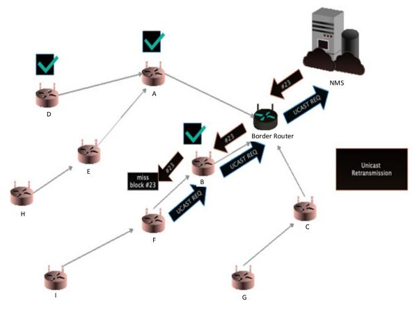
Figure 2 – Unicast Re-Transmission Progress
