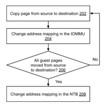
Fig. 2: Moving pages from source host to destination host
