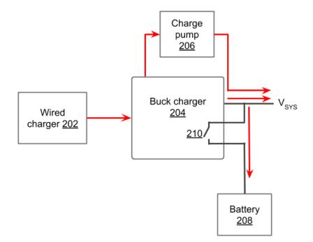
Fig. 2: Traditional combination of buck charger and charge pump
