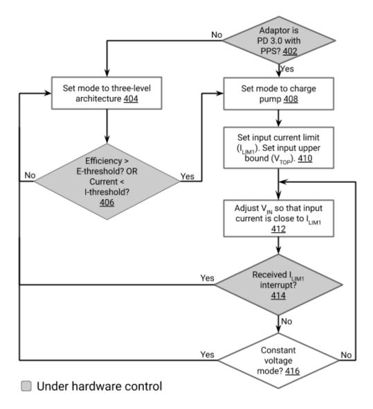
Fig. 4: Actions of the controller to switch mode between charge pump and three-level architecture
