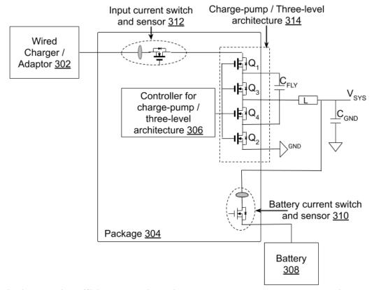
Fig. 3: Fast, high-efficiency charging using three-level and charge-pump architectures
