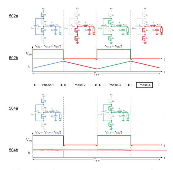
Fig. 5: Mechanism to switch modes between charge pump and three-level architecture
