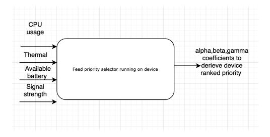
Figure 2: Calculations of the rendering coefficients by the feed render priority selector.
