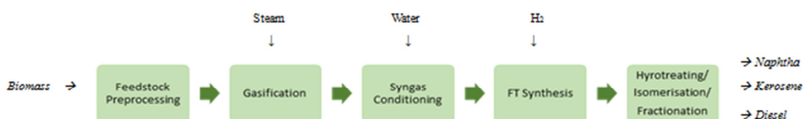
Figure 3. Biomass to FT-SPK flow diagram.
