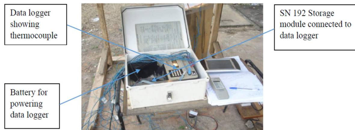
Figure 5 21X Micrologger, Campbell Scientific Incorporation, U.S.A
