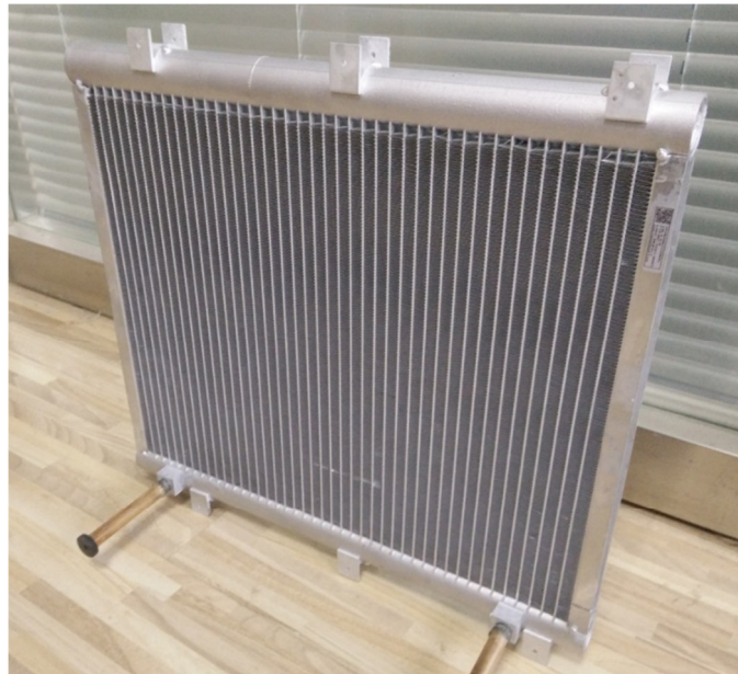
Figure 2.b: Microchannel condenser Figure 2: Photograph of the two condensers
