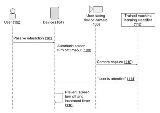
Fig. 1: Managing device screen turn off or dimming based on user attention
