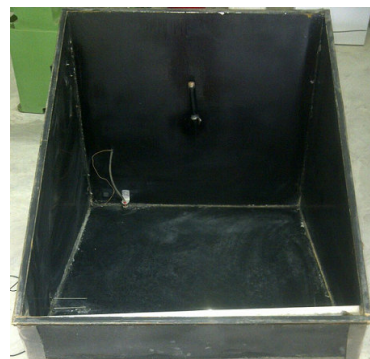
Figure (2) the galvanized body of the conventional solar still
