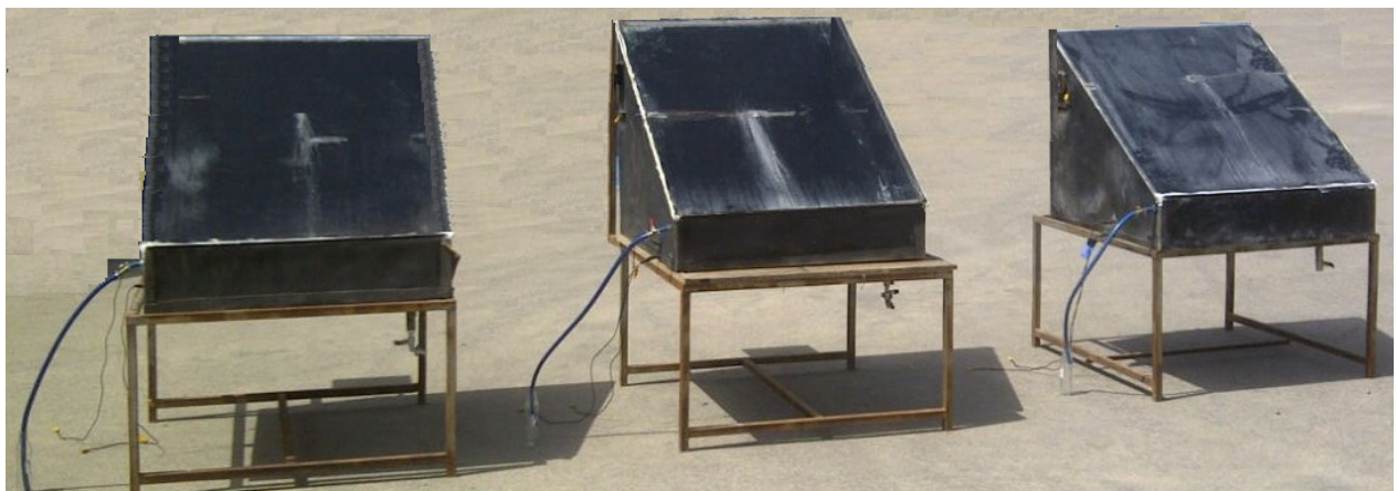
Figure (7) the three solar stills in situ
