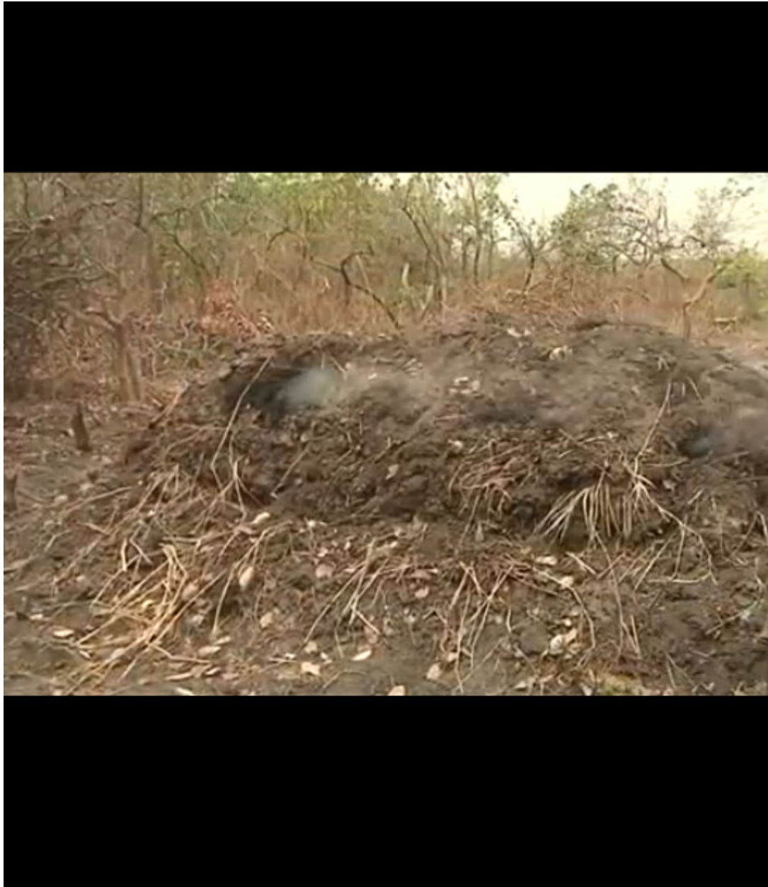
Plate 2: An earthmound kiln burning slowly Source: Field survey, 2015.
