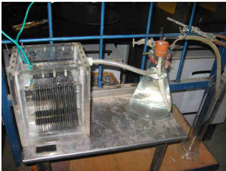
Figure 2: The setup for measuring the HHO flow rate.
