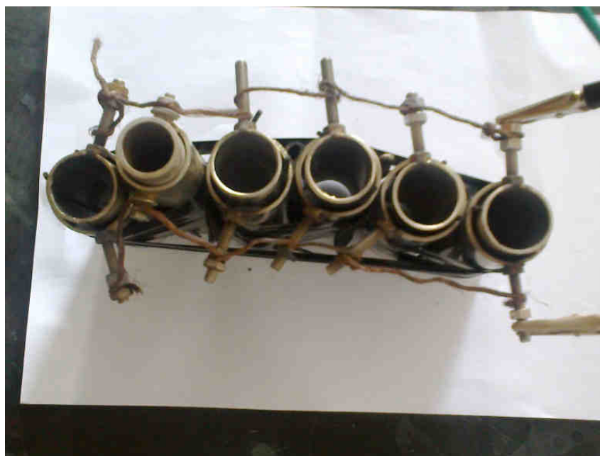
Figure 4: Cylindrical electrodes connected in parallel.
