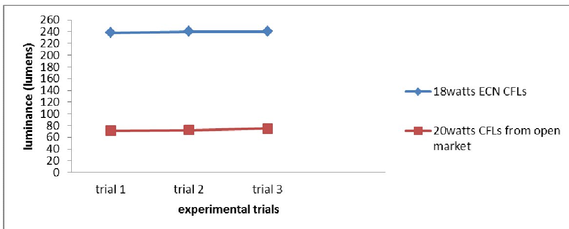
Fig 3: Results of luminance assessments for 18watts ECN CFL and 20watts CFL from open market
