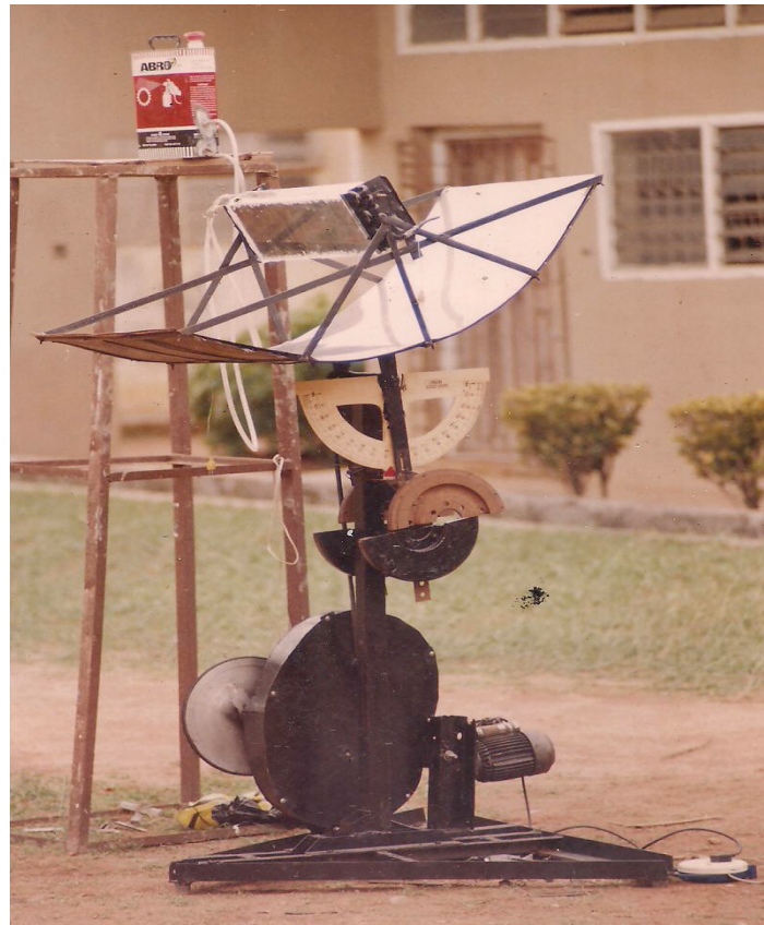
Plate 1: The tracking system set-up alone
