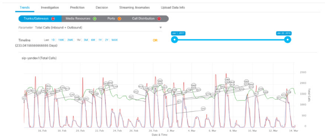
Figure 10: VCAD User Interface - Trends. Number of calls from a user on a selected trunk. This view shows the behavior over a one-month time window. The observed values are reported in blue, the predicted value reported in red, and if a moment t is anomalous, it is highlighted with a circle (on the top) and associated anomaly identifier. An anomaly susceptibility is chosen relatively high for this case.
