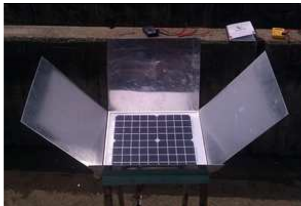
Figure 1: Solar PV panel with diffuse reflector system
