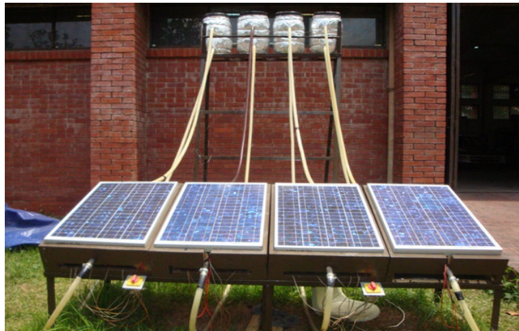
Figure 5: Photovoltaic Thermal Solar System Set-up
