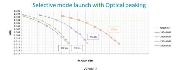
The dual-launch combination described herein is helpful to additionally enhance the supported link length at a higher data rate. It has been determined empirically that optical peaking is crucial for enhancing the link distance.
