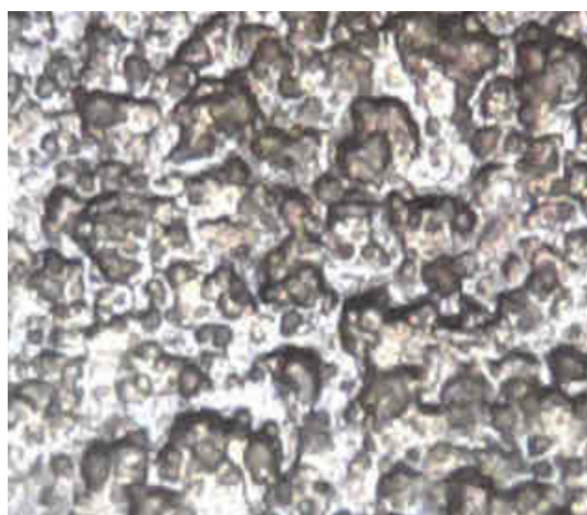
Figure 2: Optical microscopic photograph of Mg alloy after pickling in H 3 PO 4 solution (X=500)
