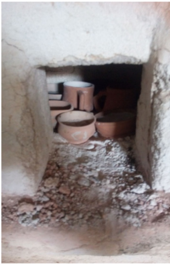
Plate 1: The crucibles were placed in the muffle kiln for firing
